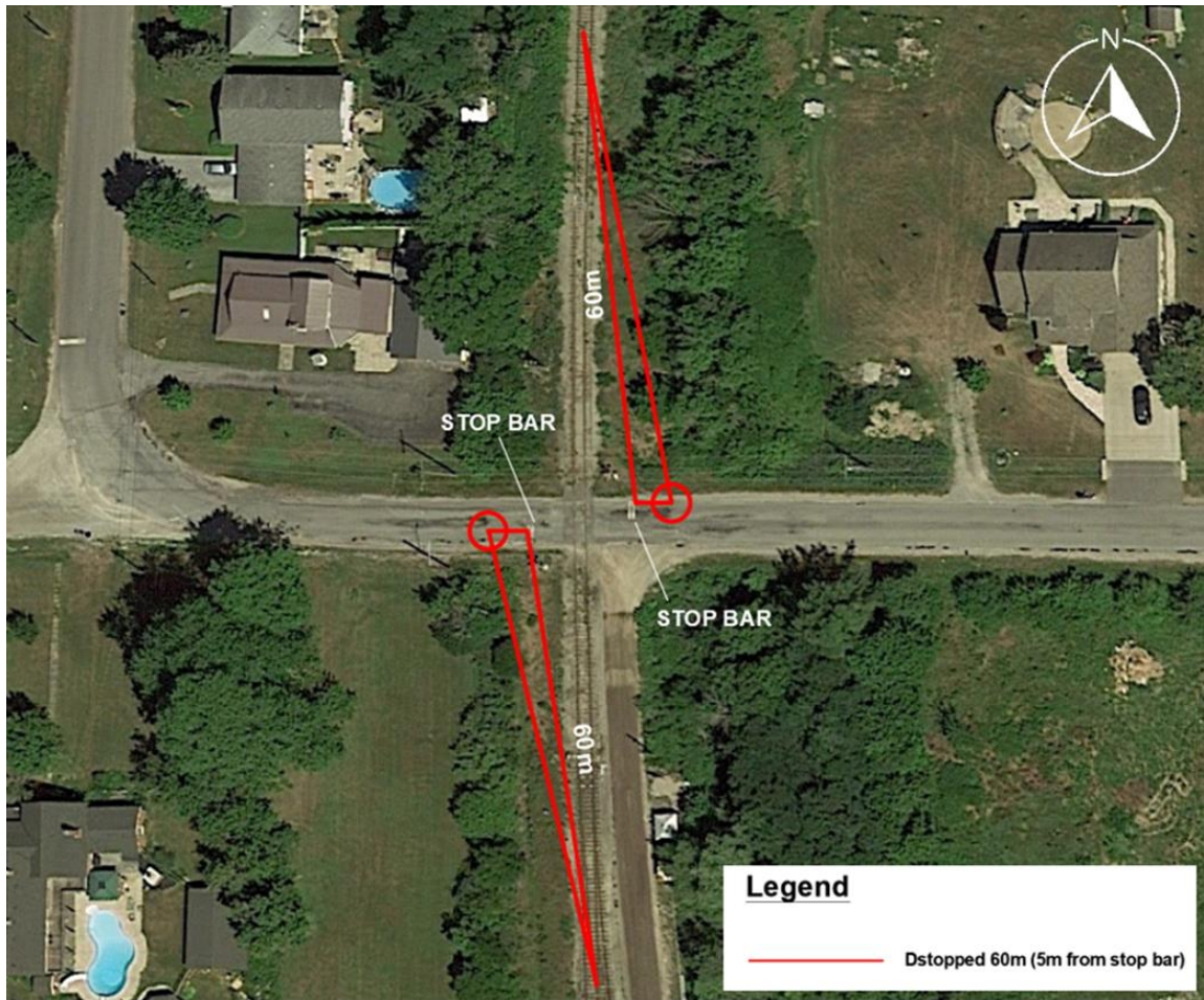
Figure 5.4 – Barron Road (W) Rail Crossing D_{Stopped}
